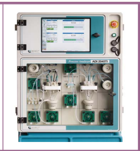
Figures 5 & 5a. Rendering of an analyzer that is closely integrated with the plating process
