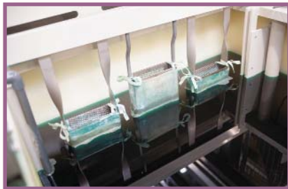
Figure 3. A typical Watts nickel bath setup.
